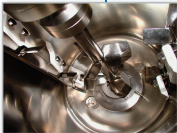
Coaxial agitator with saw disc on the bottom
