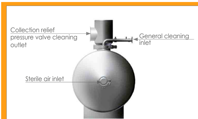
CIP solutions inlet connections
